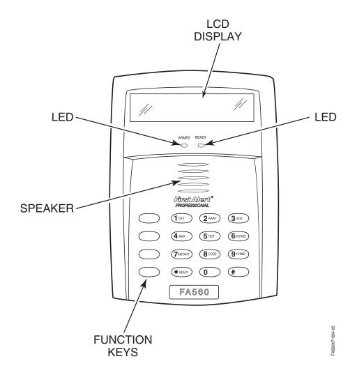
**IMPORTANT!** When using the keypad to enter codes and commands, sequential key depressions must be made within 3 seconds of one another. If 3 seconds elapses without a key depression, the entry is aborted and must be repeated from its beginning.
