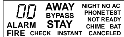
TYPICAL FIXED-WORD DISPLAY (FA260KP shown)
